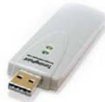
When RF Receivers are used near each other, each Receiver needs to be set on its own channel.
